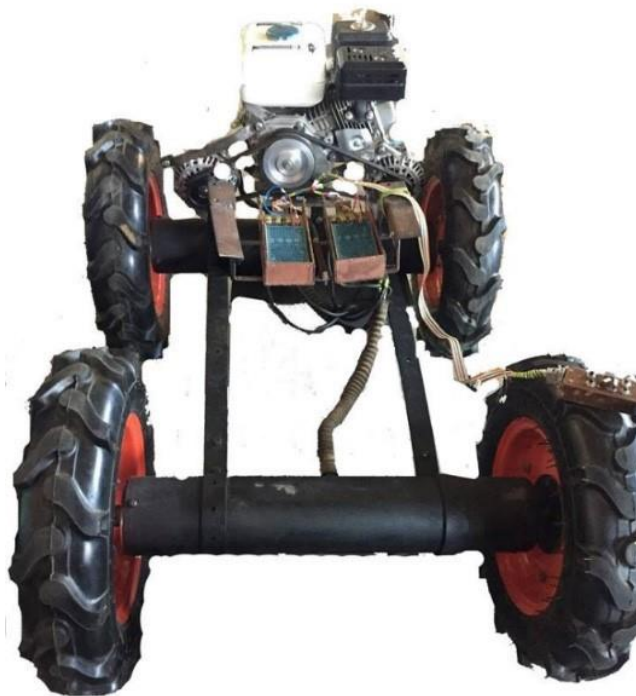
Fig.8. Placing of control blocks on the mobile machine.
